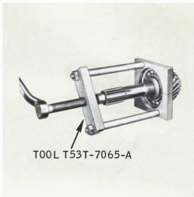
Removing Input Shaft Bearing — New Process 541 Five-Speed Transmission
