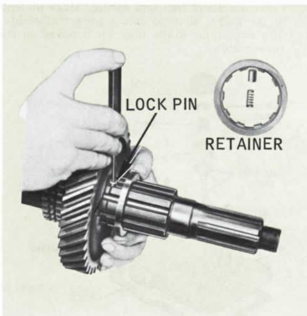
Removing Second-Speed Gear Thrust Washer — New Process 541 Five-Speed Transmission
