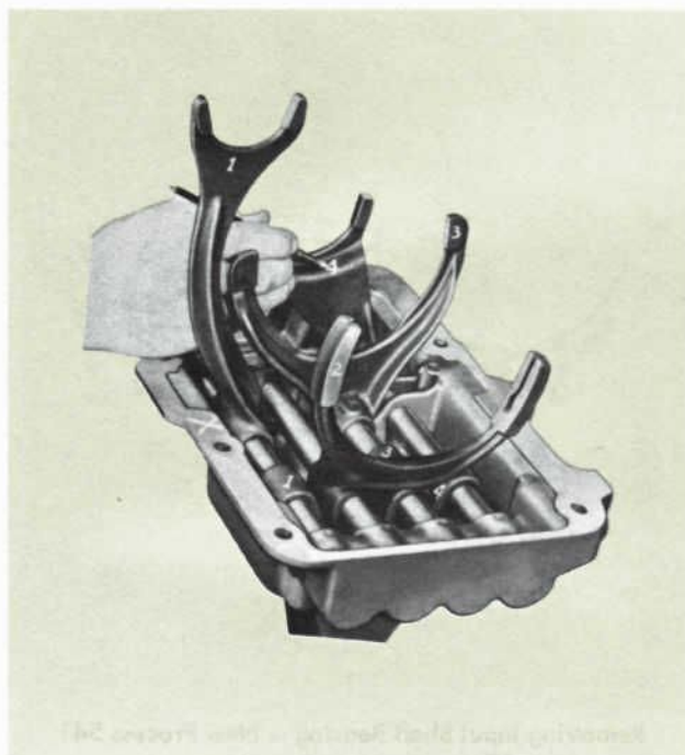
Marking Shifter Fork and Gate — New Process 541 Five-Speed Transmission
